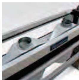
Dust exhaust hoods with four outlets.
