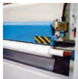
Panel thickness Control barrier with emergency stop.
