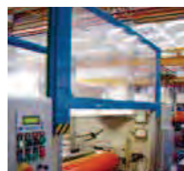
Upper protection with total visual access and prepared for gas extraction
