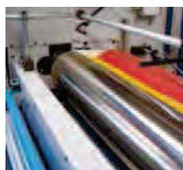
Metallic dosing roller with internal heating by thermal oil.
