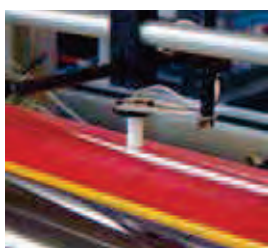
Level detectors for the glue supply control.
