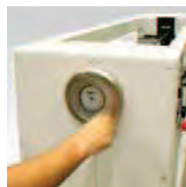
Rising through manual spindle with analogic indicator.
