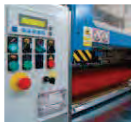
Glue grammage adjustment by speed variation.
