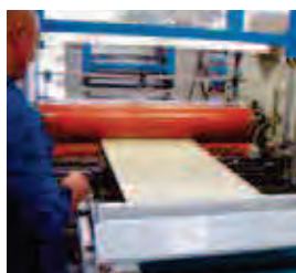
Gluing of both sides of the panels.
