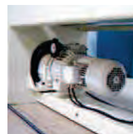
Single motor driving to the 2 or 4 pressing rollers.
