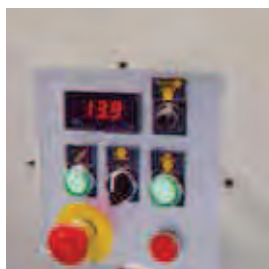
Speed regulation through INVERTER with digital display.
