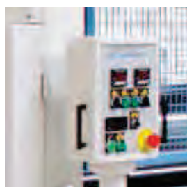
Digital Control of the roller temperature (option).
