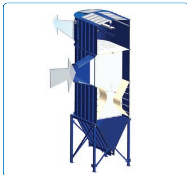
SBF filter with conical bottom and side inlet. Cross-section shows Coanda plates, used to accelerate and compress particles so that they settle to the bottom.
