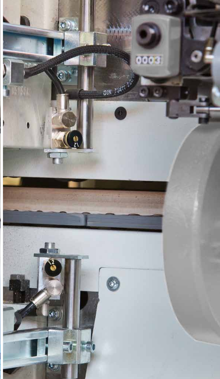
Installation example antistatic coolant spraying system in cabin, prior to the cross cut saws
