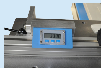
Digital read-out and large swiveling back stop
