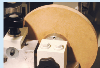
Round backing wood with 6 manual adjustable positions.
