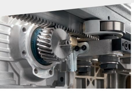
The perfectly linear movement of the tool holder carriage is achieved through a helical rack and pinion system and is driven by a brush-less servomotor.
