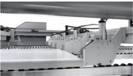
The grippers ensure the book is firmly secured. Their specific design and machine logic enable the full ejection of cut panels from the cutting line, making it easier for the operator to handle both panels and waste.
