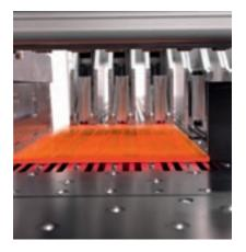
Perfect alignment of very thin and/or flexible panels, minimising cycle times thanks to the side alignment stop integrated in the blade carriage.
