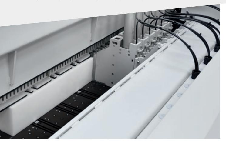
The double presser has a split, independent structure that ensures even, controlled pressure on the book of panels to be cut thanks to the absence of openings for the grippers. It creates a real airtight chamber for rough trim cuts, allowing the dust to be completely removed.
